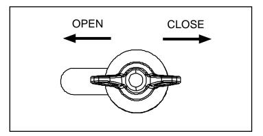
**Figure 8.29** The shutter is located on the underside of the appliance, on the right side. To adjust the shutter, loosen the wingnut. Retighten the wingnut after adjustment.
